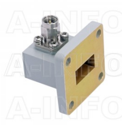
42WCA2.4M_Cu Right Angle Rectangular Waveguide to Coaxial Adapter 18-26.5GHz WR42 to 2.4mm Male
